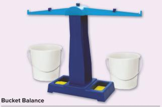
This balance features large capacity 2L buckets. Compensator clips for level and accurate measurements. Includes 5 x 1g, 5 x 5g and 5 x 10g stackable weights which can be easily stored in the bottom of the base.
