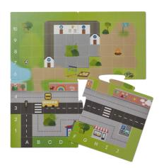
Use the Movement TagTiles® to lay down a route for KUBO to follow on the activity map. Place KUBO on the first TagTile. Make sure you align KUBO's wheels accurately to keep the robot on track. Watch KUBO move.
