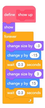
Map pin shows up at the destination after receiving the destination information: When the vehicle receives the oral command, it sends the destination information to the map pin.
