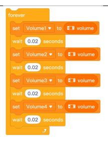
$\circ$  To continuously display sound levels, write a script as shown:
