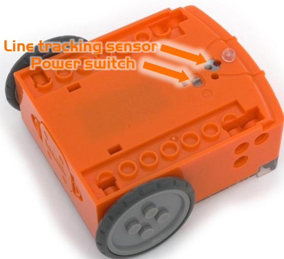
Edison's power switch and line tracking sensor
