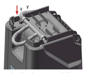
2. Place brackets over pedal bar And secure with screws
